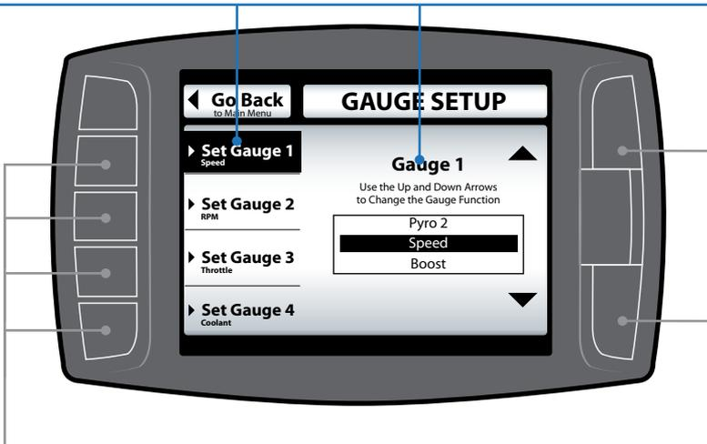
To highlight a different gauge location press the selection button that coincides with that gauge location. So to select gauge location 1, press the second button down on the left hand side of the Mini Maxx. To select the 4th gauge location press the bottom button or the 5th button down on the left side.
