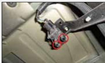
The DPF Pressure Sensor is located under the bed in front of the axle on the inside of the passenger side frame rail. You may pull the two rubber lines off of the sensor but **DO NOT UNPLUG THIS SENSOR!** Unplugging of the Pressure Sensor may result in erratic engine operation and loss of power.
