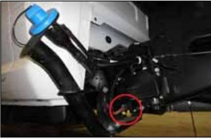
2. Slide the yellow lock-tab DOWN to dis-engage the lock and unplug the harness.
