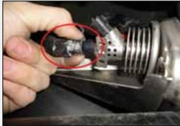
2. The main urea harness is the large black harness located near the urea injector above the urea tank. Flip the large gray locking tab to disconnect the harness.
