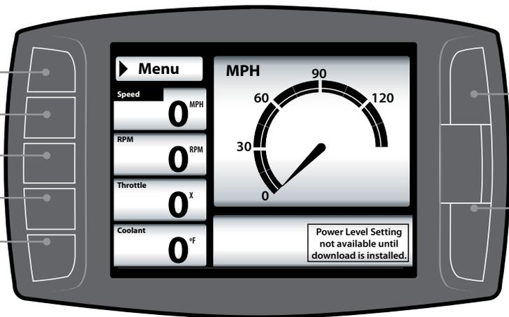
Press any of the four buttons on the left that coincide with the four vehicle parameters to display that particular vehicle parameter on the large gauge in the upper right side of the screen. Hold a button down to view the different graph types for the large gauge.
