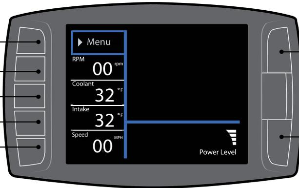
Press any of the four buttons on the left to select items on the screen that are adjacent to the button position.
