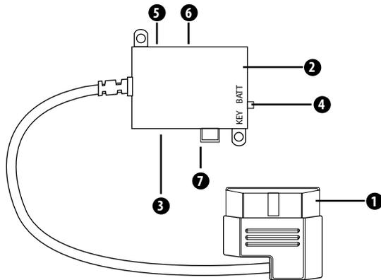
**Note:** On some vehicles it is recommended to move the OBD II port to a safer location. Because the Mini Maxx will remain plugged in, the adapter can be kicked/bumped and broken. Please move your OBD II connection to a safer location if you feel it is in a position that may allow it to get damaged.
