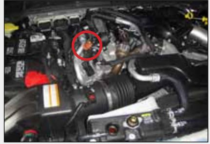
2. Unplug the EGR Butterfly Valve located near the radiator fan shroud.
